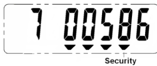
Phase Failure Count
