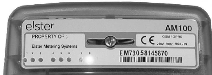
Your Smart Meter may be fitted with a modem which will allow your Service Provider to access the meter remotely via the GSM Network.
