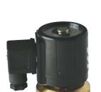
Series 3000 – General Purpose Valves, normally closed. (Energise to open) For Water, Hot Water, Air, Oil etc. Fast opening and closing Brass body with a choice of diaphragm material, Nitrile, EPDM (WRAS certified) or Viton. Electrical connection by DIN socket. Protection to IP 65s
