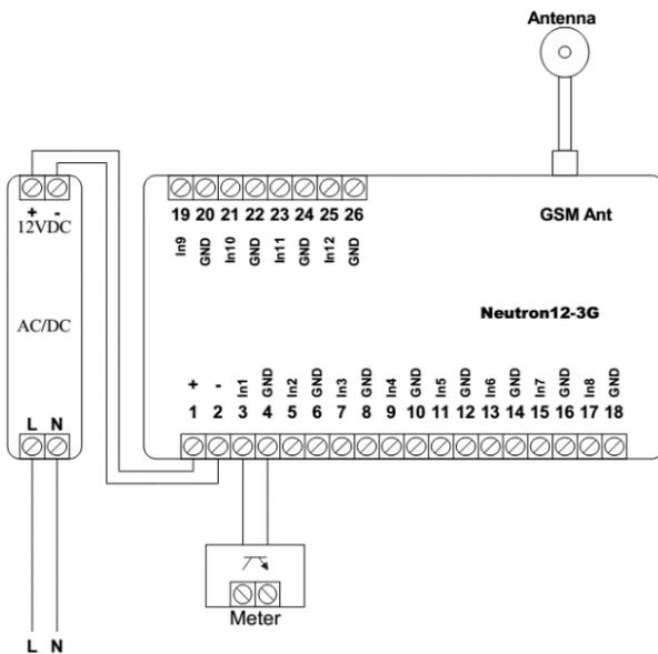
For example JAMAK 2x(2+1)x0,5mm2 instrumentation cable can be used between the meter and Neutron12-3G. The open collector or relay output of a single meter is connected to Neutron12-3G as shown above.
