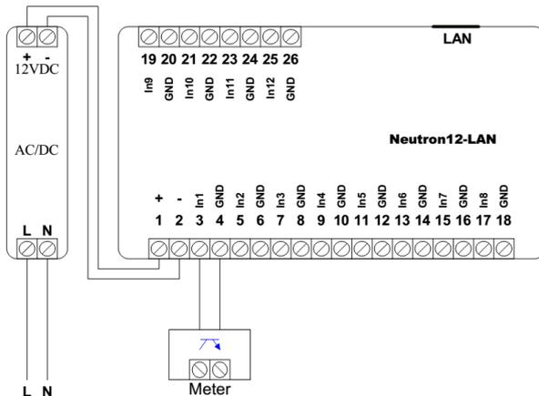
For example JAMAK 2x(2+1)x0,5mm<sup>2</sup> instrumentation cable can be used between the meter and Neutron12-LAN. The open collector or relay output of a single meter is connected to Neutron12-LAN as shown above.
