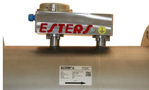
The flow meter GD 300/GD 500 can be installed in horizontal or vertical position. A condensate discharge is integrated into the measuring head, which guarantees the outflow of condensate of 100 % moist gas without sediments.
